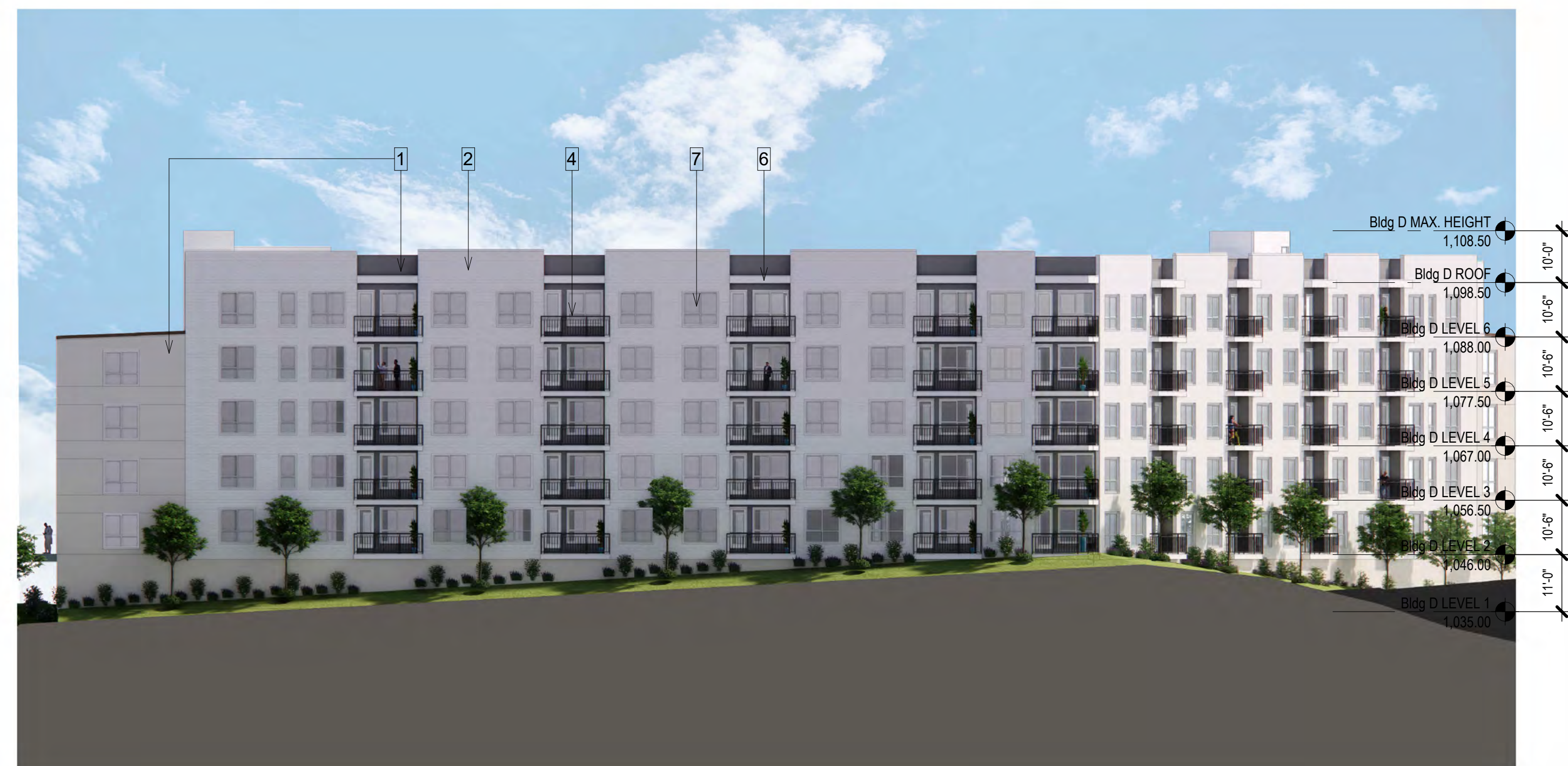
Bldg D NORTH ELEVATION SCALE: 1" = 20'-0"
